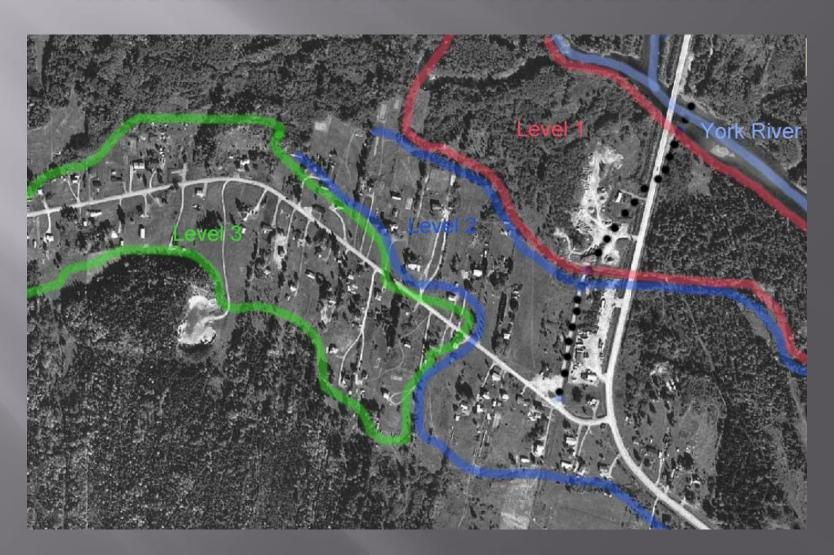
This highway blocked flood-water from moving eastward on the lowland, causing minor flooding in the low areas of level 2. Water that did rise into the fields simply crossed over the second road, thus continuing to the Bay.
